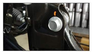
16. Re-install the brake line bracket to the strut body, but with the bracket rotated as shown in the photo. Originally the brake line was attached from the bottom upwards to the strut, now it will be mounted to the top of the strut body using the factory hardware.
