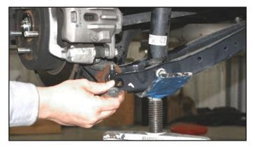
**35.Install the Rear Sway Bar Brackets to the sub**frame using the provided M8 counter sunk bolts. Apply a drop of thread locker to the threads before installing. Torque to 25 ft-lbs.
