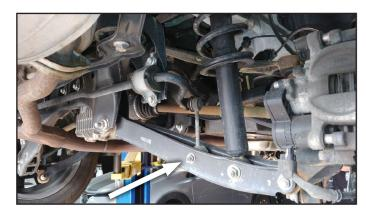
**26.** Disconnect the sway bar at the subframe and let the sway bar hang out of the way.
