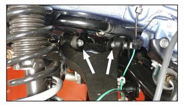
**28. Loosen but do not remove the front lower control** arm bolts.
