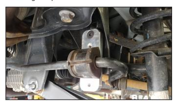
**36.** Install the sway bar to the brackets using the factory hardware and factory pinch bracket. Make sure to install the factory pinch bracket with the locking tang down. Torque to 25 ft-lbs.
