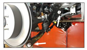
**29.** Loosen but do not remove the rear lower control arm bolt at the subframe.
