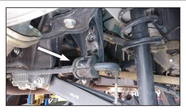
27. Loosen but do not remove the upper control arm bolts.
