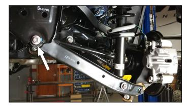
30. Support the strut and lower control arm, remove the lower strut and knuckle bolts. Lower the control arm down, while holding the strut. Remove the strut from the vehicle. A helper is recommended to hold the strut from falling.
