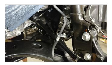
15. The cam bolt's head flange has hash marks that correspond to a notch on the strut body. Rotate the cam bolt until the hashes are facing the inside of the vehicle, and align the last hash mark with the notch. This will set camber to maximum negative. Torque both bolts to 95 ft-lbs.
