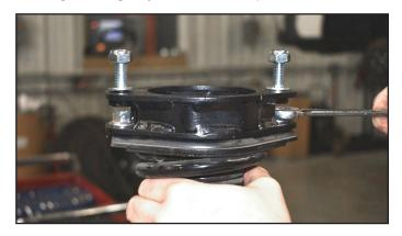
**33. Install the completed strut assembly to the car** using the provided M10 flange nuts. Do not tighten at this time. A helper is recommended.
