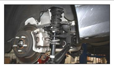
34. Raise the lower control arm into place and install the lower strut hardware. Do not tighten at this time. Use the jack and raise the lower control arm up to set pre load on the strut. Re-install the lower knuckle bolt. Torque to 95 ft-lbs.
