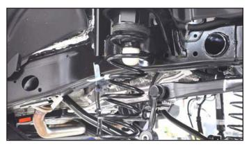
**18. Install the bump stop spacer into the lower coil** mount, using the supplied 3/8" x 3" bolt, washers, and nut through the spacer and coil mount. Tighten using 9/16" wrenches.
