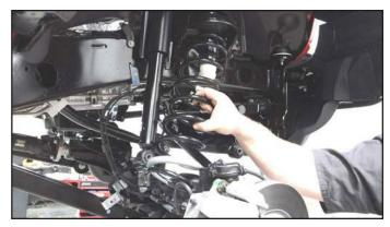
**15. Use a 10mm wrench to disconnect the brake line** bracket from the lower coil spring mount. Retain hardware for reuse.
