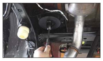
14. Install the coil spring isolator and coil spring.
