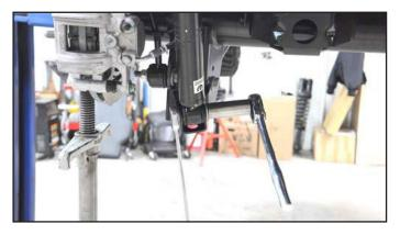
5. Use an 18mm socket and wrench to remove the lower sway bar link hardware.
