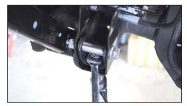
23. Use the floor jack to lift the axle housing and compress the suspension, then install the lower end of the shock into the extension bracket using the supplied 12mm x 65mm bolt, 1/2" washers, and 12mm nut.
