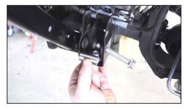
22. Tighten the lower bolt using a 9/16" socket and wrench. Torque to 30ft/lbs.
