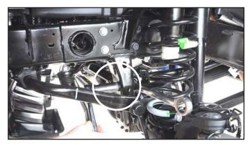
7. Use an 18mm socket and ratchet to remove the bottom sway bar link bolts. Retain the hardware for re-use.
