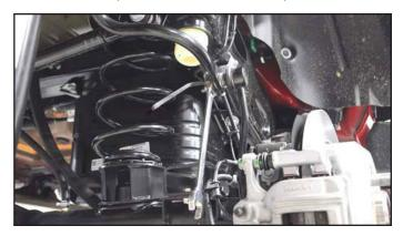
**10. Attach the supplied straight sway bar link using** the supplied 12mm x 65mm bolt, 1/2" washers (bolt head side only), and 12mm flange nut.
