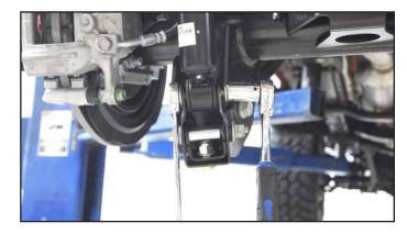
**20. Tighten the lower shock bracket bolt using a** 3/4" socket and wrench. Torque to 65ft/lbs.
