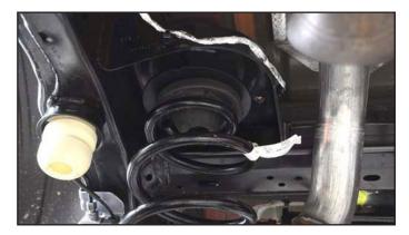
**15. Install the supplied rear shock extension brack**et using the factory shock bolt and supplied crush sleeve. Do Not Tighten.
