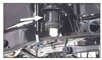
17. Re-install the coil spring.
