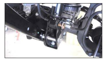
24. Tighten the factory bolt using an 18mm socket and wrench. Torque to 55ft/lbs.
