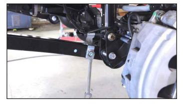
**27. Remove the sway bar link from the sway bar us**ing a 6mm hex key and an 18mm wrench.
