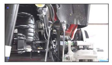
**12. Install the supplied coil spring spacer washer on** top of the coil spring pocket.
