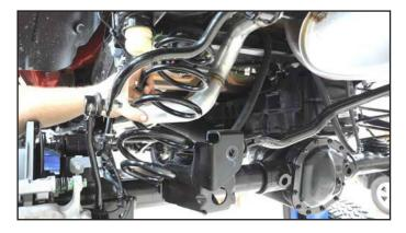
**7.** Install the supplied bump stop spacer on the axle using the supplied 3/8" x .75" bolts, washers, and flange lock nuts. (You will use 2 bolts, 2 washers, and 2 nuts per side)
