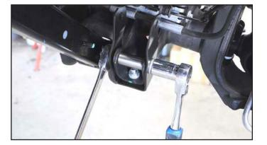
**25. Tighten the lower shock bolt using an 18mm** socket and wrench. Torque to 55ft/lbs.
