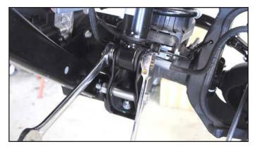
**26. Install the brake line bracket on the lower con**trol arm using the factory hardware. Tighten using a 15mm wrench. Torque to 18ft/lbs.
