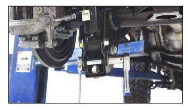
**19. Tighten the lower shock bolt using an 18mm** socket and wrench. Torque to 55ft/lbs.
