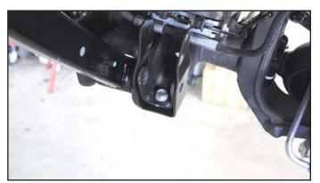
**21. Place the supplied crush sleeve into the factory** shock bracket. Install the factory shock hardware into the brackets and through the sleeve.
