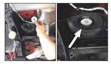
**13. Install the supplied rear coil spacer, using the** supplied 1/2" x 2.5" bolt. Tighten using a 3/4" socket. Torque to 65ft/lbs.
