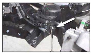
**16. Install the supplied spring spacer with coil spring** isolator under the spacer.
