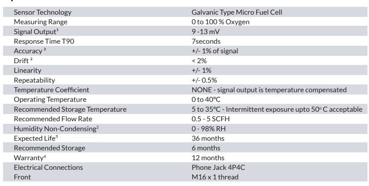
**Note:** SRX-CT-3 is designed as a component for breathing air equipment, user must verify its compatibility with intended equipment. For optimal accuracy, sensor must be calibrated before each use and after 24 hours of continuous use in oxygen above 90%. Do not expose sensor above 50°C for extended period of time. Failure to do so may have negative impact on its performance and life.
