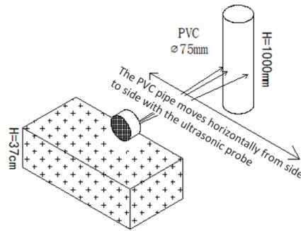
② The tested object is a "corrugated box" perpendicular to the 0° central axis, with a length \* width of 60cm\*50cm.
