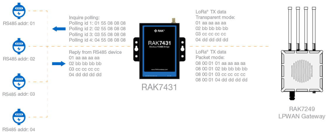
Figure 2: RAK7431 WisNode Bridge Serial polling mode
