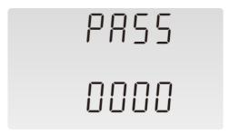
Setting up is password-protected so you must enter the correct password before processing. If an incorrect password is entered, the display will show: PASS Err
