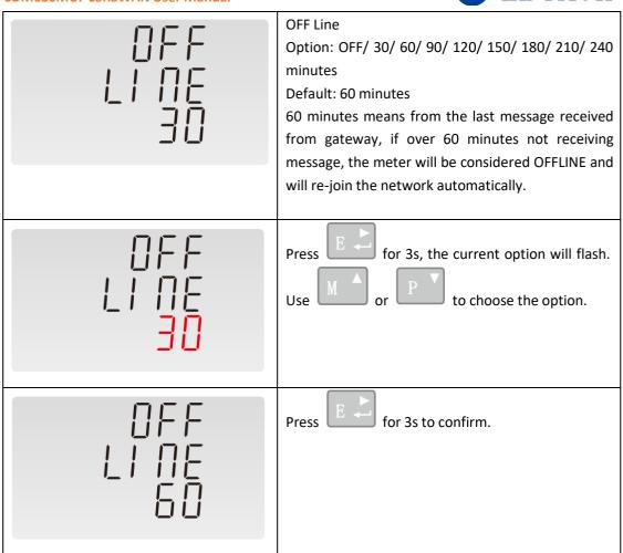
**NOTE:** Under the active upload mode, the OFF Line time should be set to a value bigger than the active upload interval time.
