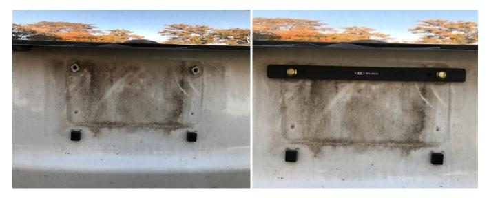
Step 1: Install the BLOX license plate adapter using (2) of the supplied bolts. You will install them on to the outer location
