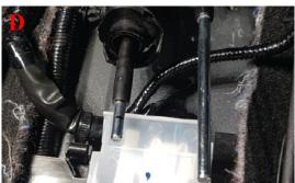
Slide the supplied steel ball cups onto the cables and tighten the grub screws. Loctite is recommended here on each screw.
