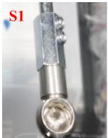
Place the two base bars on the threaded holes and screw them on with the supplied countersunk screws, we recommend a small drop of screw adhesive such as Loctite per screw. The longer 90mm bar on the front and 80mm bar for the rear.
