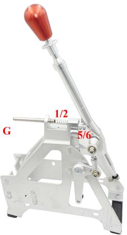
To adjust the shift travel, first determine the desired center position of the shift lever and tighten the lower spring stop under the shift bracket using a 5 mm Allen key. The shift lever should be slightly tilted to the left.
