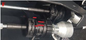
Place the shifter on the latches and tighten the 4 nuts.
