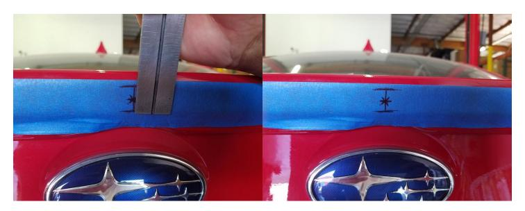
Step 3: Using the straight ruler, measure 3/8" from the bottom of where the 3/4" flat space begins. Mark with pencil or pen. In case the marks do not meet, please measure again.
