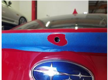
Step 5: Drill a 25/64" hole. Remove some tape around this hole.
