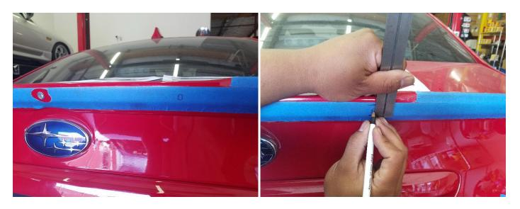
Step 9: While the Gurney Flap is temporarily mounted at the center, trace the remaining holes with a pencil or pen. The remaining hole-centers will be measured using the same methods and steps just completed in locating the center hole.
