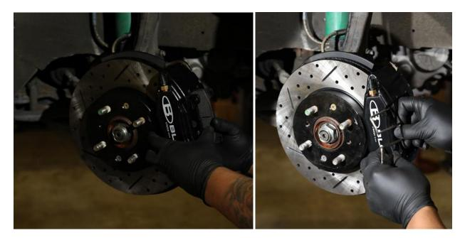
Step 5: Slide the new BLOX Racing brake pads into place. Make certain that the friction material is facing the rotor. Install the brake pad retainer clip. Connect brake hose.
