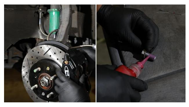
Step 4: Mount the new BLOX Racing front caliper. Use "red" Loctite® 271 on the bolt threads. Torque to 60 ft/lbs.
