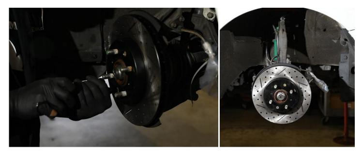
Step 3: Place the new BLOX Racing front rotor on to hub, making sure it sits and fits flush against the axle hub. Make sure rotor slots are facing correct direction.
