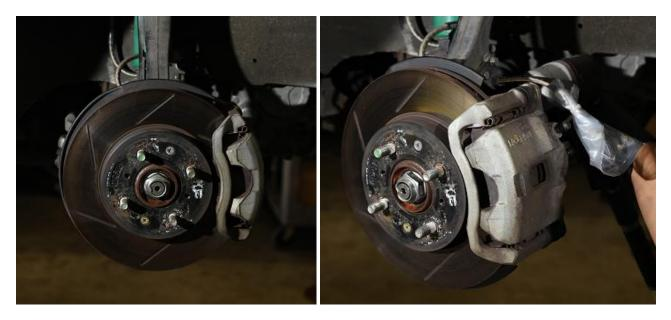
Step 1: Disassemble the brake system by removing the calipers and lines. It is recommended that the lines be replaced with new or steel braided hoses.
