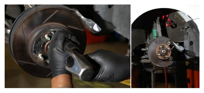
Step 2: Disassemble and remove the brake rotors. Remove any material from the hub faces. Clean the areas with brake cleaner or degreaser.
