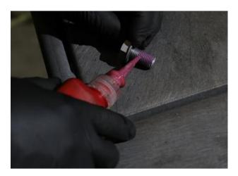
Step 4: Mount the new BLOX Racing front caliper. Use "red" Loctite® 271 on the bolt threads. Torque to 60 ft/lbs.
