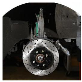
Step 3: Place the new BLOX Racing front rotor on to hub, making sure it sits and fits flush against the axle hub. Make sure rotor slots are facing correct direction.
