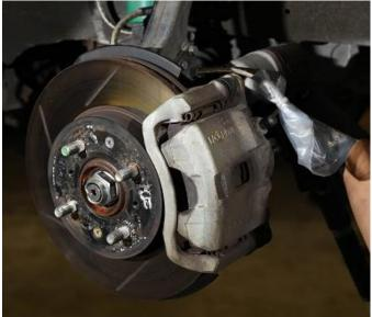
Step 1: Disassemble the brake system by removing the calipers and lines. It is recommended that the lines be replaced with new or steel braided hoses.
