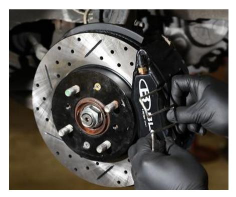
Step 5: Slide the new BLOX Racing brake pads into place. Make certain that the friction material is facing the rotor. Install the brake pad retainer clip. Connect brake hose.
