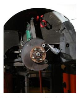
Step 2: Disassemble and remove the brake rotors. Remove any material from the hub faces. Clean the areas with brake cleaner or degreaser.
