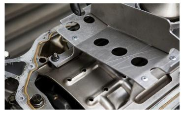
12. Locate the oil baffle and install over studs, washers and retainers. Carefully slide the large opening over the oil pick up. There is no need to disassemble the actual baffle. It is secured by rivets.
