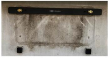
Step 1: Install the BLOX license plate adapter using (2) of the supplied bolts. You will install them on to the outer location
