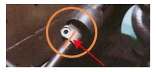
3. Loosen the bolts on the subframe. DO NOT REMOVE THE BOLTS. Drop the subframe 8mm from the chassis of the vehicle.
