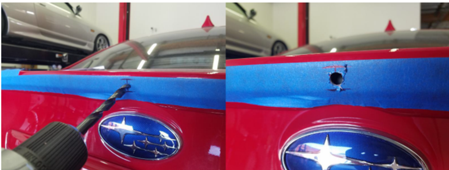
Step 4: Once you have confirmed the center, please drill a 1/8" hole at the center mark. This will help in the next step in drilling out the actual hardware mounting hole.
