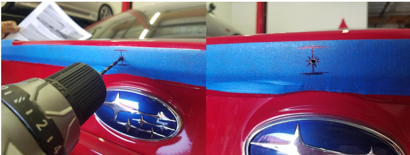
Step 4: Once you have confirmed the center, please drill a 1/8" hole at the center mark. This will help in the next step in drilling out the actual hardware mounting hole.
