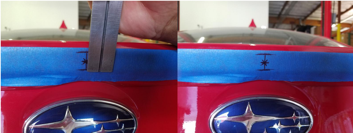
Step 3: Using the straight ruler, measure 3/8" from the bottom of where the 3/4" flat space begins. Mark with pencil or pen. In case the marks do not meet, please measure again.
