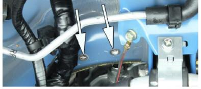
Install the provided rivet nuts, using the above images as a reference on how to assemble the rivet nut, M6 bolt and washers. Use the provided rivet tool. You will feel some resistance at first before it gets easier to tighten.
