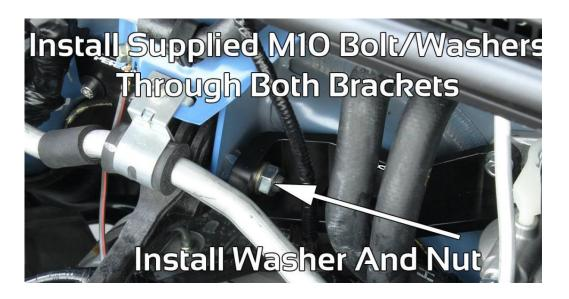
Tighten the M8 bolts and nuts on the left plate to 15ft/lbs-18ft/lbs. Fold back or cut off the firewall cover.
