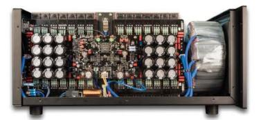
Board layout itself is not the sole factor in the prodigious capability of the SAE 2HP-D. Kessler, who has been designing solid-state amplifiers for over 50 years, specified the use of innovative ThermalTrak output devices. With ThermalTrak, the temperature sensor required for the amps' bias tracking is actually built into the same package as the output transistor. This allows accurate real-time bias and
