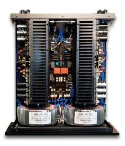
Inside, each channel has a custom-wound toroidal transformer with hand-selected low-noise core and independent secondary outputs with one for each half of the two bridged output stages feeding independent rectifiers and a bank of 12 3900  $\mu$ F filter capacitors for total power supply storage of 93,600  $\mu$ F per channel. Further, the capacitors are located as close as possible to the amplifier outputs to reduce power supply resistance and further improve performance.
