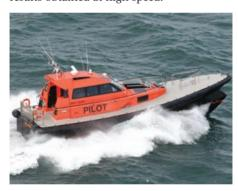
In addition, this feature imparts inherent roll damping qualities, only moderately slowing as the beak bow pierces the next wave.
