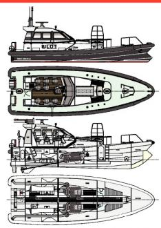
waterline and a wave-piercing beak bow to minimise pitching. Twin turbo-charged diesel engines rated at 450kW drive fixed pitch propellers, enabling a 25-knot operational speed with good fuel efficiency.
