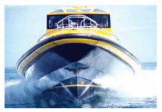
The 'Kestrel's' beak bow lowers into the water in rough weather via the vessel's trim tab system. This lowering adjusts the longitudinal trim to increase speed and decrease drag
