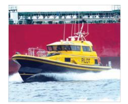
In the wake of the disaster, PPSP searched abroad for the best pilot boat design for operation in frequently treacherous conditions, settling on France-based Pantocarene's ORC concept and bringing it to Hart Marine. Sporting its now-distinctive beak bow, the resulting new-generation selfrighting vessel displays excellent sea-keeping capabilities in the worst weather conditions and sea states.
