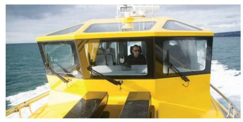
To reduce pilot fatigue, the vessel's resiliently mounted wheelhouse features vibration dampening aualities as well as noise levels below 70 decibels
