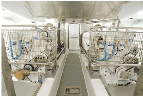
The vessel is powered by twin 600hp Cummins QSM II diesel motors.
