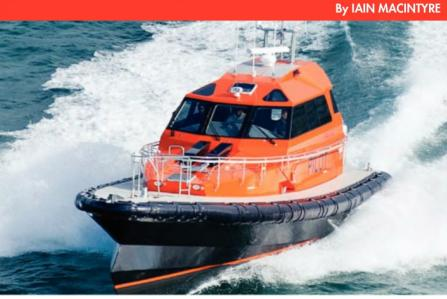
with self-righting capability, every design element of the vessel came under the naval architects' scrutiny. The shape and line of the hull, together with an integrated fendering system, helps minimise the risk of the "venturi effect", a phenomenon that can 'suck' pilot boat hulls to the side of a large ship at speed.
