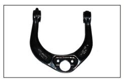
Photo 1. Cast arm with bushes removed.
