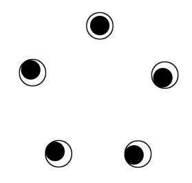
The best procedure is to tighten each lug by hand whil wriggling the wheel to ensure that the lugs seat properly in the wheel. Do this a little at a time. If you have to use a lug wrench (or ratchet), just be sure that you very light on the tightening so that if the wheel is off-center, the other lugs can pull it back to center as they are tightened.
