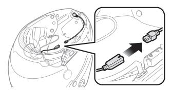
Note: The shortest cable is for the microphone.
