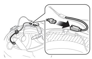
**Note:** The shortest cable is for the microphone.
