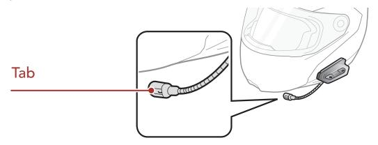
5. Align the arrows on the main unit and microphone cables and insert the microphone cable into the microphone connector.
