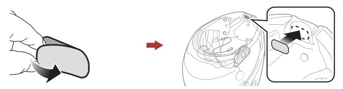
2. Attach the wired microphone to the hook and loop fastener for wired microphone.
