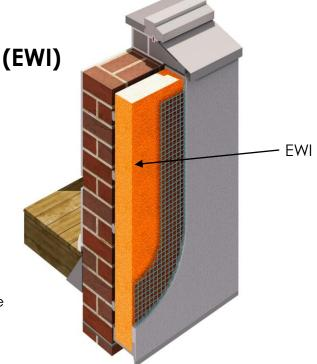
Jablite EWI HP+ is manufactured from expanded polystyrene (EPS) and can be bonded or mechanically fixed to an external wall. It can be used in conjunction with a variety of render and cladding systems including timber or plastic weatherboarding, tile hanging and reinforced-render systems.
