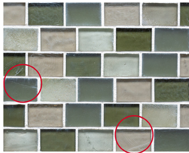
Muse, shown above, has some fissures on the surface, and on this example, the grout has been partially cleaned from the fissures.
