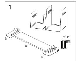
Shelf includes one shelf board (A), two brackets (B), 4 large wall screws (C), 4 small screws (D) and bins when ordered.
