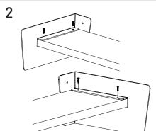
Position right and left brackets (B) on shelf board (A) sides. Pre-drilled holes on board should face bracket holes. Secure board with small screw D.
