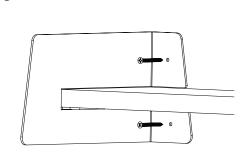
Slide Shelf includes hardware for securing shelf to **drywall only**. Use proper hardware for your specific case and follow hardware manufacturer instructions.
