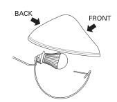
Install so that the BACK of the shade (the one closest to the shades peak) is on the lamp holder side.
