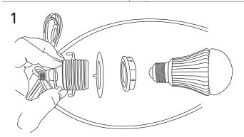
Screw the metal ring so that it sits halfway into the threaded lamp holder. Place the lamp holder through the ring of the lamp frame. Screw the plastic ring to secure the lamp holder to the frame. Make sure the wire sits under the frame.
