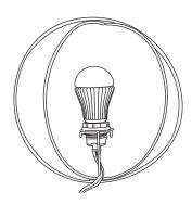
Bottom view of correct cord placement and lamp holder assembly.
