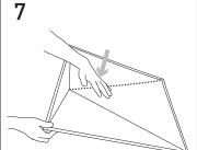
Gently fold inward to release tension in the creases. This will allow the tile to sit flat in the drop ceiling grid.
