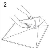
Carefully fold side flap as shown to prevent wrinkling or damage to tile.
