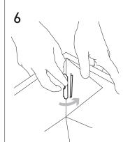
Secure tab by inserting into the second slot and fold over edge.
