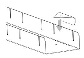
Insert caster covers as shown lining up the holes on the plate cover and the base.
