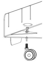
Secure plate covers by inserting the caster through the holes and securing them with the washer, lock washer and nut (in that order)
