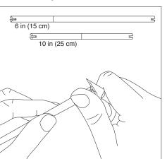
STEP 1 Mark the 24 in (60 cm) dowel 6 in (15 cm) from the end and the 20 in (50 cm) dowel 10 in (25 cm) from the end. CAREFULLY cut notches in the ends of the dowels.
