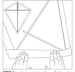
**STEP 4** Lay the frame on top of Loop. Cut the material so that it is 2 in (5 cm) larger than the frame. Fold the edges of Loop over the frame and secure with carpet tape. Fold the corners in and reinforce them with tape.
