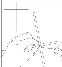
**STEP 2** Cris-cross the dowels at the markings you made earlier and wrap the string around them in an X pattern to secure them. The notches should be parallel to the ground.
