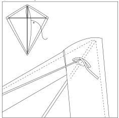
**STEP 5** Make holes using a needle to secure a 24 in (60 cm) piece of string from the top corner to the bottom. Tie the remainder of your string to this line (this will be your flying string)\*.
