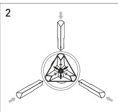
Carefully flip seat hub unto a clean and soft surface to prevent scratching. Insert legs into hub pockets until legs align with hub.
