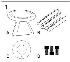
Glide Stools include one seat hub (A), three legs (B), one leg locking washer (C) and three 1/4 20 hex screws (D)
