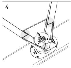
Leg shoulders should meet edge of the hub and small leg notches should be aligned to hub pocket openings as highlighted above.
