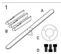
Fly Seesaw includes one plank hub (A), three legs (B), one leg locking washer (C) and three 1/4 20 hex screws (D)
