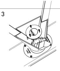
Secure legs using the leg locking washer and 1/4 20 screws. Use a hex key (not included) to secure the locking washer. **Do not over tighten.**
