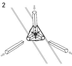
Carefully flip plank hub unto a clean and soft surface to prevent scratching. Insert legs into hub pockets until legs align with hub.
