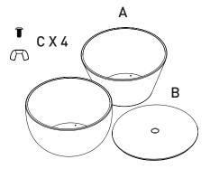
Flip Stools include Cones / Bowls as ordered (A), seat lid (B) and 4 screws and wing nuts (C) 1
