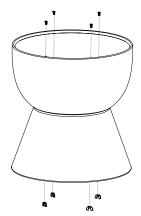
Secure Cones / Bowls using the screws and wing nuts as shown. Insert the screws from the shape / side that will be the seat top.
