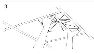
Rotate tiles at an angle to insert into ceiling grid. Position the tile perimeter so it sits flat on the grid. Tiles on the edges can be cut with a sharp utility knife or power tools. Mark with masking tape for accuracy.
