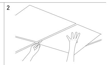
If replacing old ceiling tiles, remove the tiles and ensure the grid is clean, secure and square.
