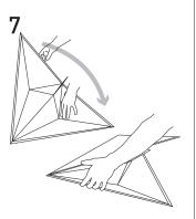
Start to fold tile over, making sure not to let the edges bow. Fold over to release tension in the creases. This will allow the tile to sit flat in the drop ceiling grid.
