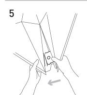
Insert tab into the edge slot.
