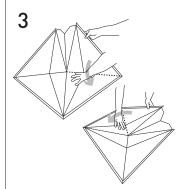
Carefully fold along the other axis. Do not apply excessive force or the tile will crease. **Repeat** on other side.
