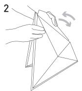
Carefully fold the locking tab as shown to prevent wrinkling or damage to tile.
