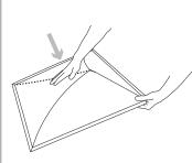
Gently fold inward to release tension in the creases. This will allow the tile to sit flat in the drop ceiling grid.
