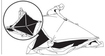
**4** Extend the bars inside the Oztent Screen House and secure them in the pockets at the bottom. After, pull out the guy ropes and peg them down at a rough 45 Degree angle to secure your Oztent Screen House.
