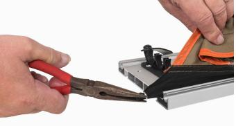
• Retain the Spring 'O' Clip attached to the end of the sail-track spline (as illustrated above). Although not an essential part, it does assist in minimizing movement of the Awning Skin and assists in removing the Skin if it needs to be replaced in the future. Reapply this clip to the end of your replacement Skin prior to reinstallation.
