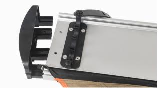
To replace the Large End Cap, simply push the replacement unit into the Main Backing Extrusion and insert rivets to secure. Note that it may be necessary to gently tap the part into the extrusion with a rubber hammer or similar.
