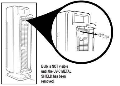
5. The UV-C Bulb is reinstalled by sliding it, horizontally, back into the slots at the top of the unit.
