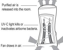
\*It is recommended to run the GG1000 continuously. Opening doors and/or windows in the room may affect the performance of the device.
