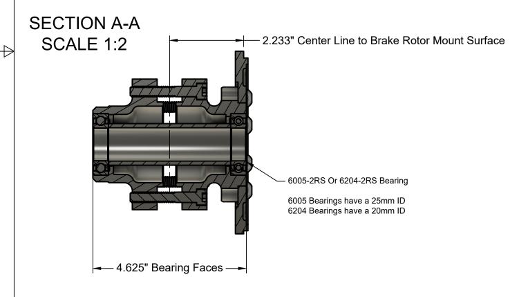
This hub assembly was designed to work with 2003 - 2004 R6 front forks, brake caliper, and rotor, when assembled with **7.750**" spread triple clamps.
