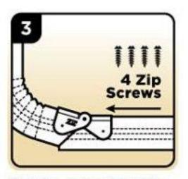
Slide the cut section of the downspout extension into the Zip Hinges™ and secure with zip screws.
