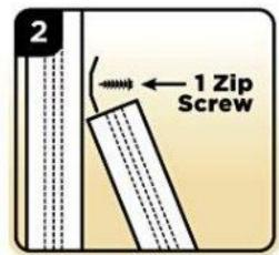
Use zip screw or 1/8" rivet to attach clasp 3/4 inches above raised extension.
