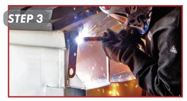
Tack weld the right arm back plate to the edge of the container, as shown above.
