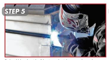
Tack weld the other side of the pipe to the right arm, as shown above.
