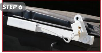
Once you are happy with the movement of the container lock, weld firmly into place.
