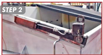
Tack weld the 100565 to the banding with the front tab flush to the front banding, as shown above.
