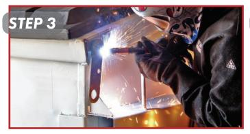
Tack weld the right arm back plate to the edge of the container, as shown above. Make sure it is welded in the same position as the left side.
