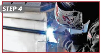
Using the front of the container as your level, cut the 1" O.D. pipe the exact length you need, and tack the pipe to the right arm as shown above. Make sure that the arms are vertical, allowing the pipe to move up and down freely.
