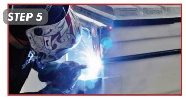
Tack weld the other side of the pipe to the left arm, as shown above.
