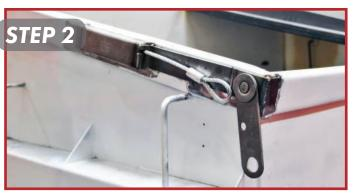
Start by welding the front of the tab, which should be parallel to the banding. Tack weld the 100555 to the banding with the front tab flush to the front banding, as shown above.
