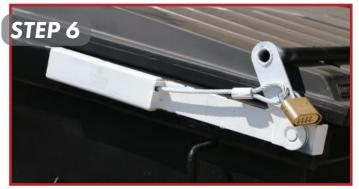
Once you are happy with the movement of the container lock, weld firmly into place. The cable loop, bar lock arm, and padlock should have a very tight fit. You want to ensure the end of the cable loop meets up with the bar lock arm and tension can be felt when applying the padlock.
