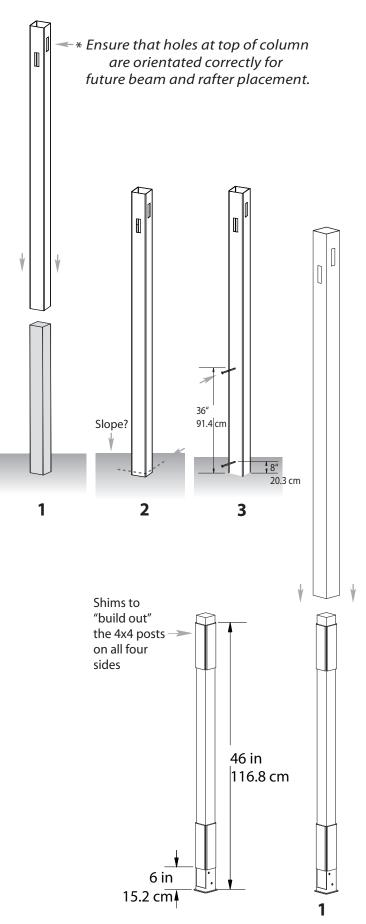
At this stage, the columns should be properly installed as per the following illustration, with the columns 78 in (198.1 cm) apart. Also, notice that the holes at the top of each post should be facing the same direction.
