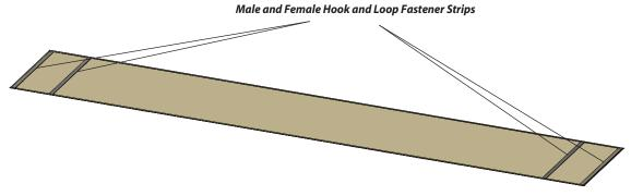
With the hook and loop fastener strips facing up, weave the canvas through the shade slats as shown. Note the pattern of the weave (below two shade slats, and above two shade slats). Starting with below two shade slats, and ending with the same.
