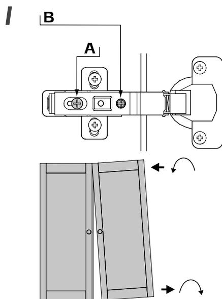
Adjusting the gap between the doors. Loosen screw 'A' slightly. Turn Screw 'B' clockwise to move the door away from the side, turn anti-clockwise to move the door towards the side. When gap is equal tighten screw 'A'.
