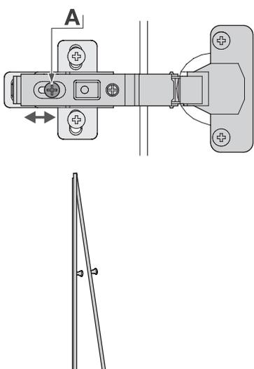
Adjusting the angle of the door. Loosen screw 'A' and slide the hinge arm either forwards or backwards until the door is vertical then tighten screw 'A'.
